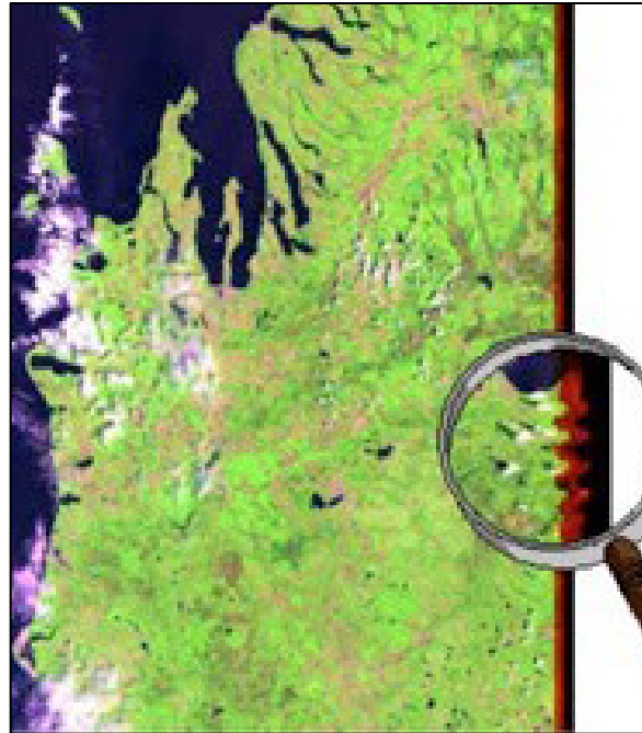
Figure 2-10. ETM+ GXA Data Anomaly caused by an X-Band Antenna Across-Track Slew Maneuver
