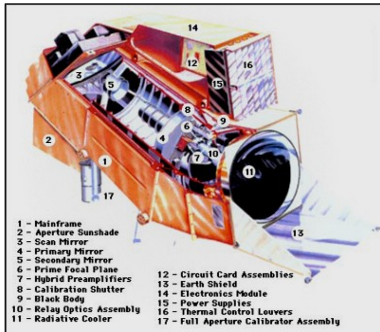
Figure 2-5. Cutaway View of ETM+ Sensor and Its Major Components
